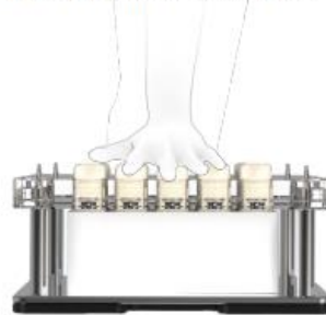
STEP 2 Place the deflector over the tray.
