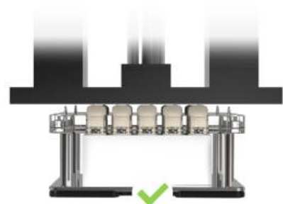
STEP 6 Press with machine to seal off the filled devices.
